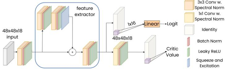
The structure of the **final feature extractor** and the **critic** and **actor** heads utilized on top of M-PPO.
