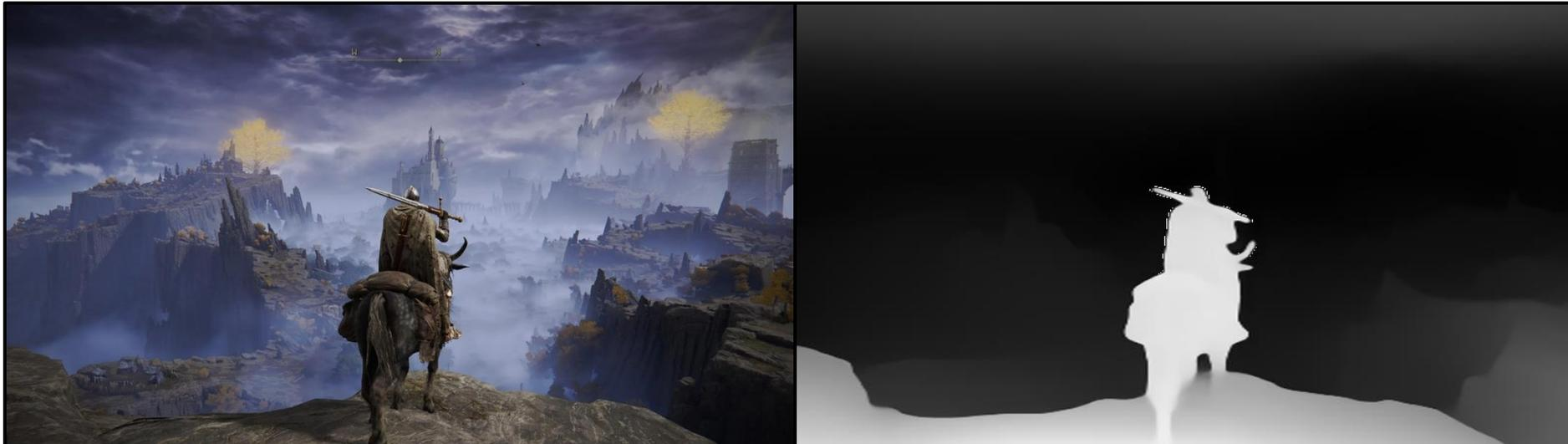
The demo uses **DPT** (Dense-Prediction Transformer) showcasing its versatility in estimating depth on any 2D image that represents a projection of a 3D scene.
